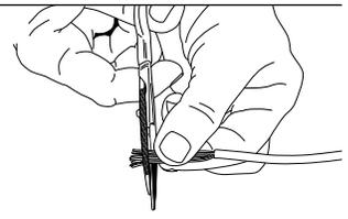
6) Slide the connector onto the wires snugging it up to the jacket. **Cat5e:** Be sure to insert cable jacket beyond the primary strain latch to ensure twists are less than 1/2" from the point of termination. **Cat6:** Be sure to insert cable jacket all the way up and behind the contacts to assure twists are less than 3/16" from the point of termination.
