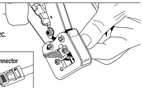
7) Crimp and trim the connector in one EZ process with P/N 100054 or 100062C.
