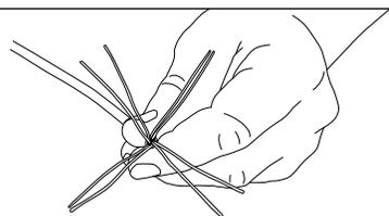
5) Determine whether you will be using the T568A or T568B configuration (above) and organize wires accordingly. Line up your wires and make a clean cut across all 8 conductors with P/N 10517 leaving approximately 1.5" of wire protruding from the jacket.
