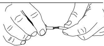
3) Separate pair ends at tip. Place your free pair separator over one of the conductor ends of each pair and push/rotate in opposite direction of the twist, separating each pair.
