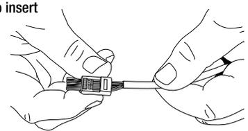
7) Crimp and trim the connector in one EZ process with P/N 100054 or 100062C.
