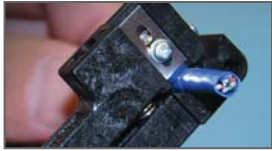
Score cable with stripper Cat. No. 45-165
