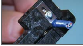
Score cable with stripper Cat. No. 45-165
