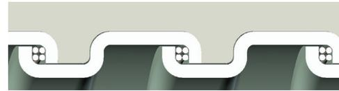
Square-Locked Design with cord packing 3/8" through 1-1/4"
