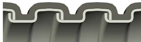
Square-Locked Design 3/8" through 2"
