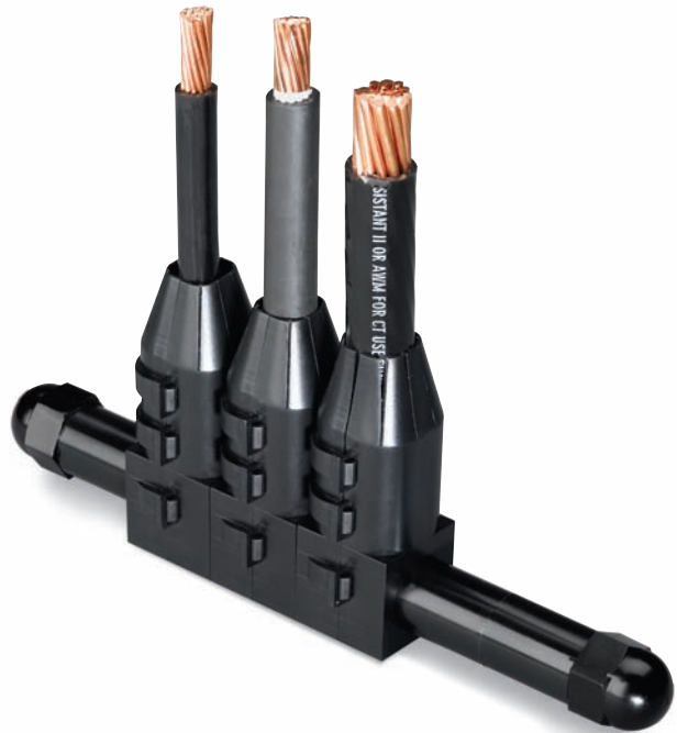
This Multi-Tap installation connects 4/0, 1 and 2 AWG cables using MD40F-3, MD1F-3 and MD2F-3 connectors with REC-3 insulators on an R3-6 rod.
