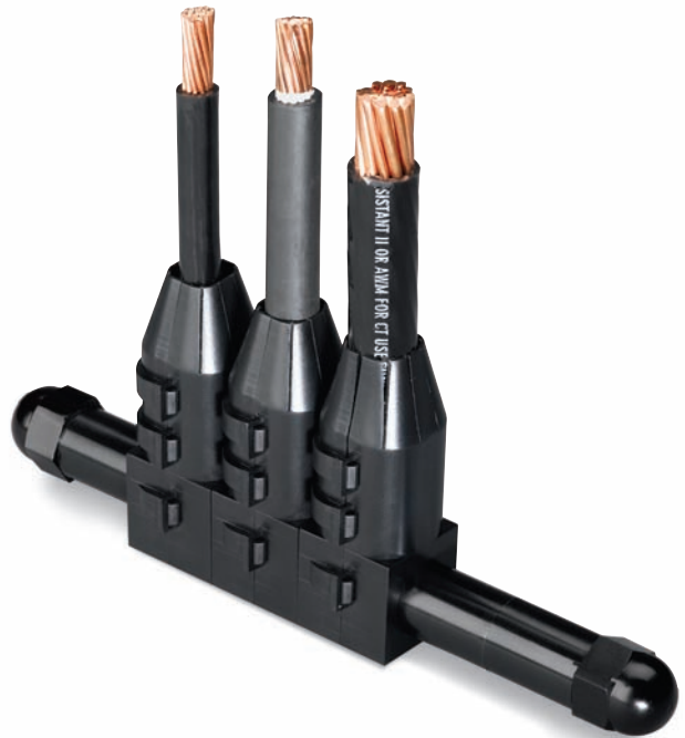
This Multi-Tap installation connects 4/0, 1 and 2 AWG cables using MD40F-3, MD1F-3 and MD2F-3 connectors with REC-3 insulators on an R3-6 rod.
