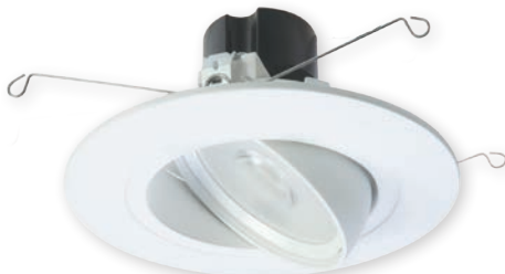
RA56069xxWH 5"/6" adjustable gimbal, 90 CRI, very wide flood
