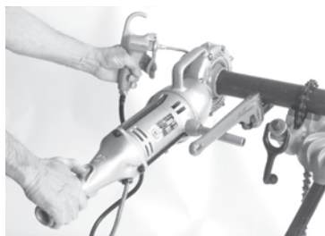
Threading using a pipe wrench as a support arm
