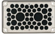
F3A-D Cellular rubber pass-through flange, 40 cables Ø 10-13 mm, 4 cables Ø 17-21 mm, 2 cables Ø 27-30 mm
