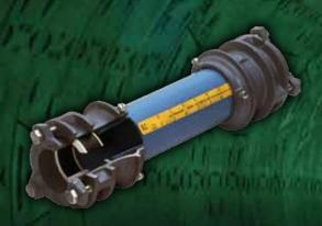
Conduit or cable entries into a facility should not function as waterways. Thruwall and floor seals offer the best defense against moisture and serve as the optimum choice for below grade foundation conduit/ cable entry. They are designed to provide a watertight blockage between poured concrete and the fitting body as well as a pressure-tight seal around the penetrating end.
