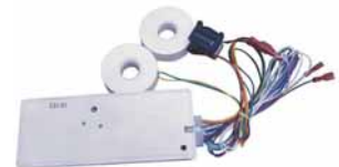
Two Element Meter
