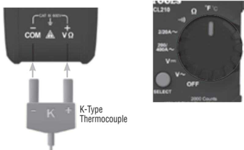
**⚠ Remove thermocouple before switching meter to other measurement functions.**
