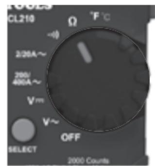
**NOTE:** When in a Resistance setting and the test leads are open (not connected across a resistor), or when a failed resistor is under test, the display will indicate O.L. This is normal.
