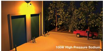
NOTE: Typical mounting heights are 10'-30'. Simulation rendering using AGi32 software.
