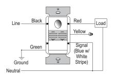
Signal wire connects to neutral. Signal wire can connect to ground in replacement or retrofit application
