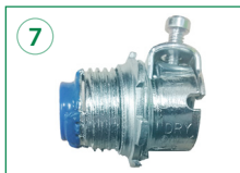
Size: 3/8": P/N E00-054-000 1/2": P/N E00-055-000 Type: Set Screw, Squeeze Material: Steel Insulated: Yes
