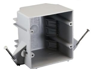
EZ32DN EZ BOX is a 32 cu. in., 2-gang, nail-on, electrical switch and outlet box for residential or light commercial new construction (new work) electrical installations. It features 8 wire clamps and enhanced angled nails for EZ installation.
