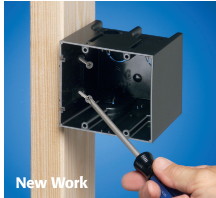
1 Attach ONE-BOX to wood or steel stud with captive installation screws. If box is too far forward or back, back the screws out to reposition.
