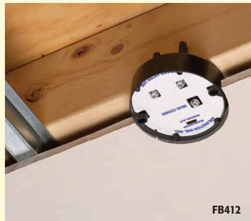
1 The FB412 fan/fixture box is perfect for 1/2" or 5/8" drywall with 3/4" furring strips or hat channel with a single layer of drywall...
