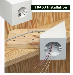
Cut a 2x8 approximately 18" long. Install FB450 on 2x8 allowing it to extend 8 to 10" past the box. Keep bottom of box level, short side of box touching angled rafter. Nail or screw assembly to rafter.
