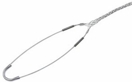
Bus drop, Closed mesh, Single eye. Cable diameter - 0.700-0.850", Bale length - 9", Mesh length - 8.5", Break strength - 1,900 lbs.
