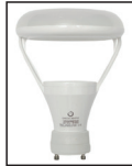
(1) 11 Watt GU24 base LED lamp/2700 Kelvin Warm White/>90CRI/750 lumens/68 LPW/ ENERGY STAR 2.0 certified/25,000 hours rated average life.
