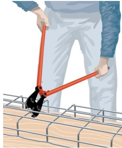
Figure 3-66 Cutting with Bolt Cutters
