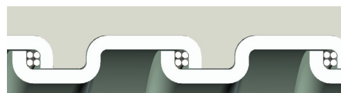
Square-Locked Design with cord packing 5/16" through 1-1/4"
