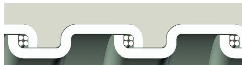
Square-Locked Design with cord packing 5/16" through 1-1/4"
