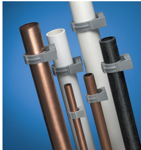
2-1/2" - 4" Press pipe into QuickLATCH, up to the first notch to lock it in place. Finish by squeezing tabs together for a super-secure hold.
