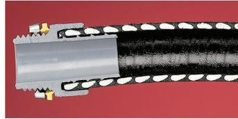
Conduit threads onto ferrule and up inside the outer body. The inside taper squeezes down on the outside of conduit for a superior liquid-tight seal. The cut portion of the conduit does not show, giving a more attractive finished appearance. Also for use with flexible non-metallic tubing. These connectors screw on easily by hand and are removable with pliers.
