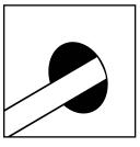
Step 1: Drill appropriately sized hole (9/16" for RFG1, 1" for RFG2) and install the cable.
