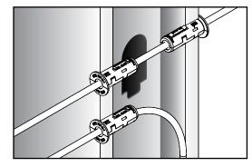
Note: For through penetrations where cable breeches both membranes of wall, a firestop grommet is required on both sides of a wall.
