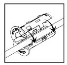
**Step 2:** Place two halves of firestop grommet around cable and snap together.
