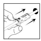
**Step 3:** Firmly push grommet into wall opening to lock in place.
