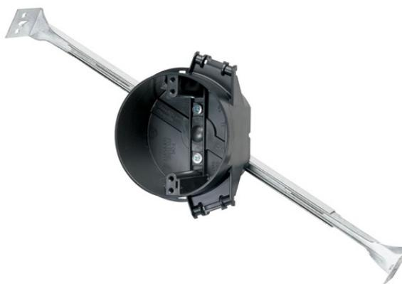
4" Round Ceiling Box with a bar hanger that adjusts to 16" or 24" joist spacing. It has four Auto/Clamps. It is constructed with impact-resistant Noryl thermoplastic, making it virtually unbreakable and non-conductive. Its depth-mounting gauge at bottom of bracket helps you align the box at the proper depth relative to the ceiling. 50 pack.
