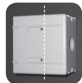
Slider plate retracted sets box in fully adjusted forward position for maximum wall substrate thickness of 1-3/8".
