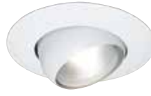
RT602GW/AT/FS Socket Supporting Gloss White Step Baffle with White Ring, Airtight, Friction Springs, for Floating Medium Base Socket Uses BR/PAR30 Lamps Order Code: 77564
