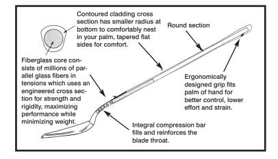
The shovel and grip ends are larger to provide leverage and control while the center tapers to help your hand slide when "slinging" the material away from the hole.
