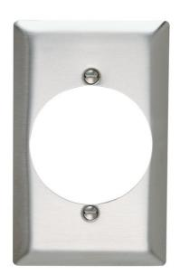
One Gang Power Outlet Receptacle Opening, 2.156" hole for 2.125" diameter device - 2 mtg. holes, Smooth Metal.
