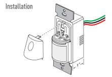
Extremely shallow (1") back housing and 6" flying leads facilitate quick installation in standard wall box
