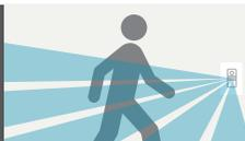
Passive Infrared technology detects heat emitted from a human body in motion and relies on a clear line of sight.
