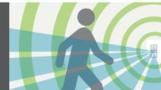
Combines PIR and Ultrasonic technology for hard to sense spaces when maximized sensitivity is required.
